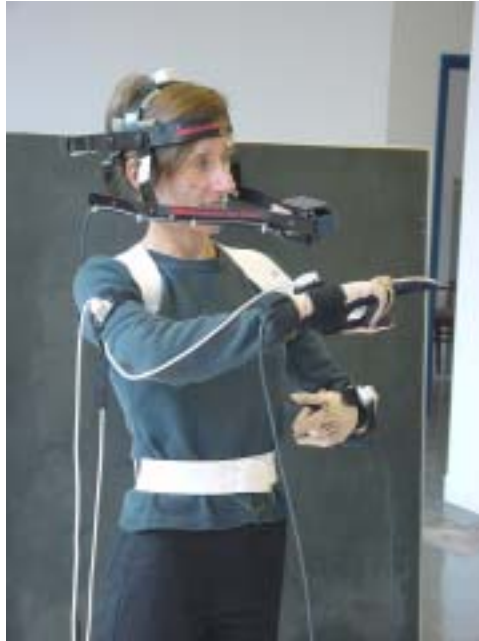
Figure 3: Data capture: face tracking camera with facial reflectors, Cybergloves for tracking the digits and Polhemus sensors taped onto the back of each hand, upper arm, body and head to track the body.
