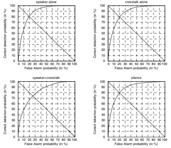
Figure 2: ROC performance curves for each crosstalk category's optimum feature set. Log energy has been excluded from the set of potential features. Diagonal lines indicate equal error rates.
