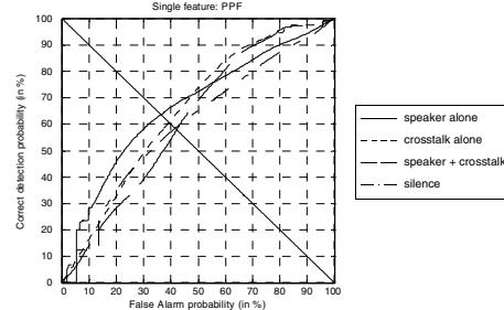
Figure 3: ROC performance curves for each crosstalk category using PPF. Diagonal line indicates equal error rates.
