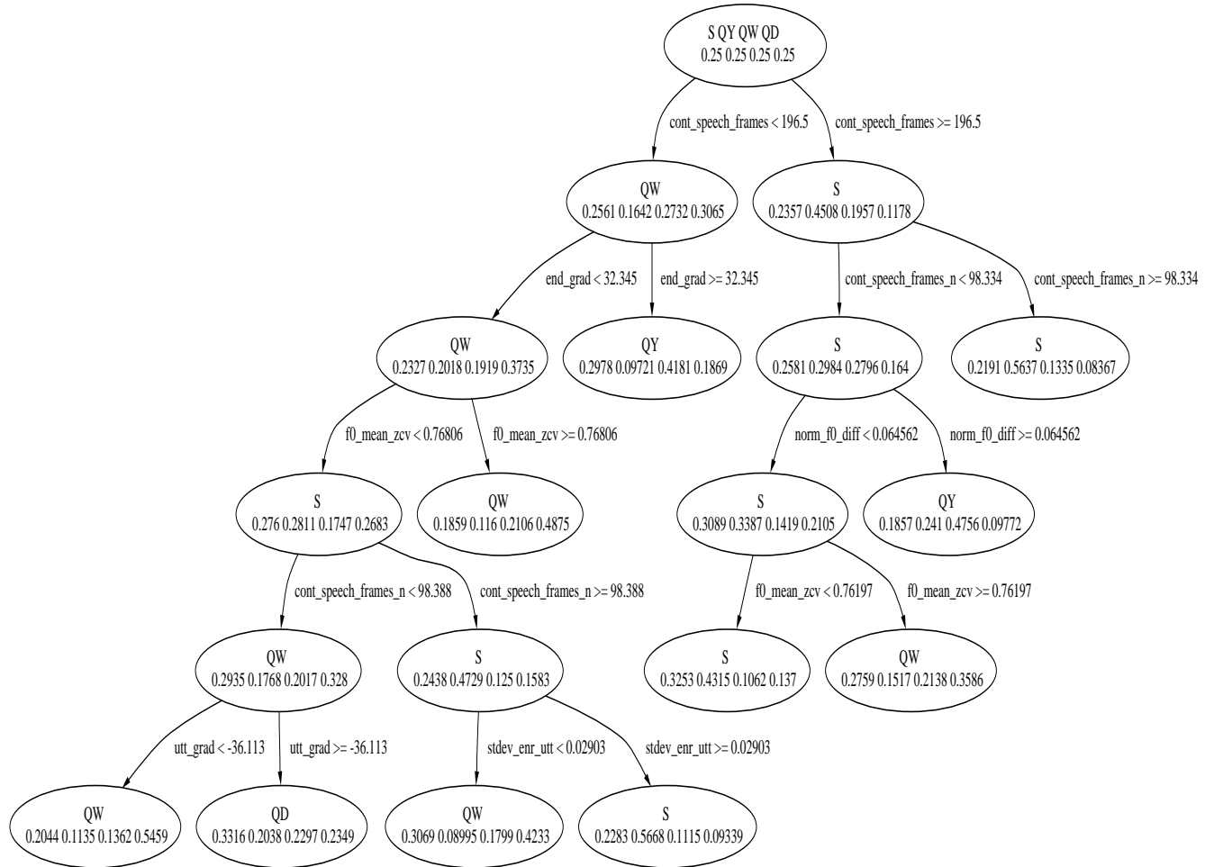
Figure 6: Decision tree for the classification of statements (S), yes-no questions (QY), wh-questions (QW), and declarative questions (QD)
