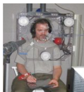
Figure 1. Carstens' new 3-D sensor 'cube'. The transparent plastic box surrounds a participant's head, creating a comfortable experimental experience which enables data collection sessions of 1 hour and more.
